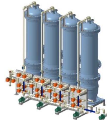
Adsorption columns for Pilot Plant
