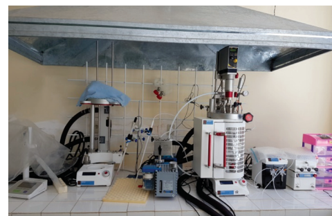
Reactor tipo Laboratorio ATLAS SYRRIS AUTOMATED SYNTHESIS
