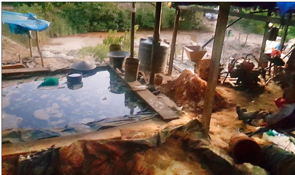
Photo 11 Purification pool to obtain amalgamated gold.
