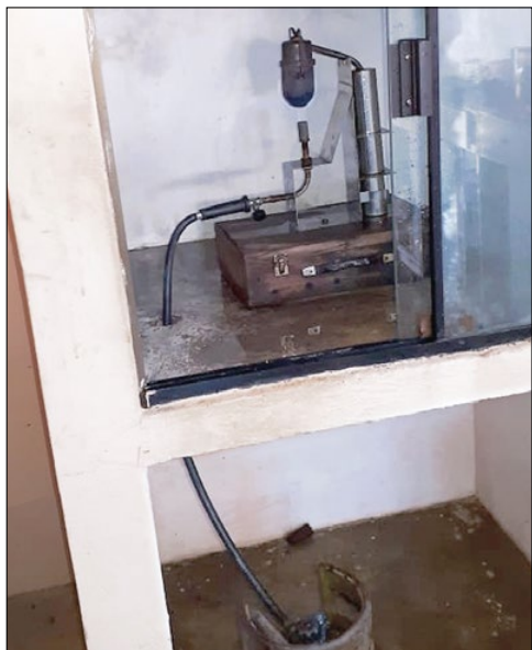
Photo 10 One kg container of “El Español” mercury and a retort burner equipment.
