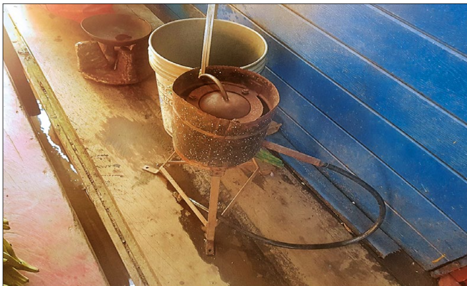
Photo 20 Burning equipment for amalgamated gold - retort (2019).
