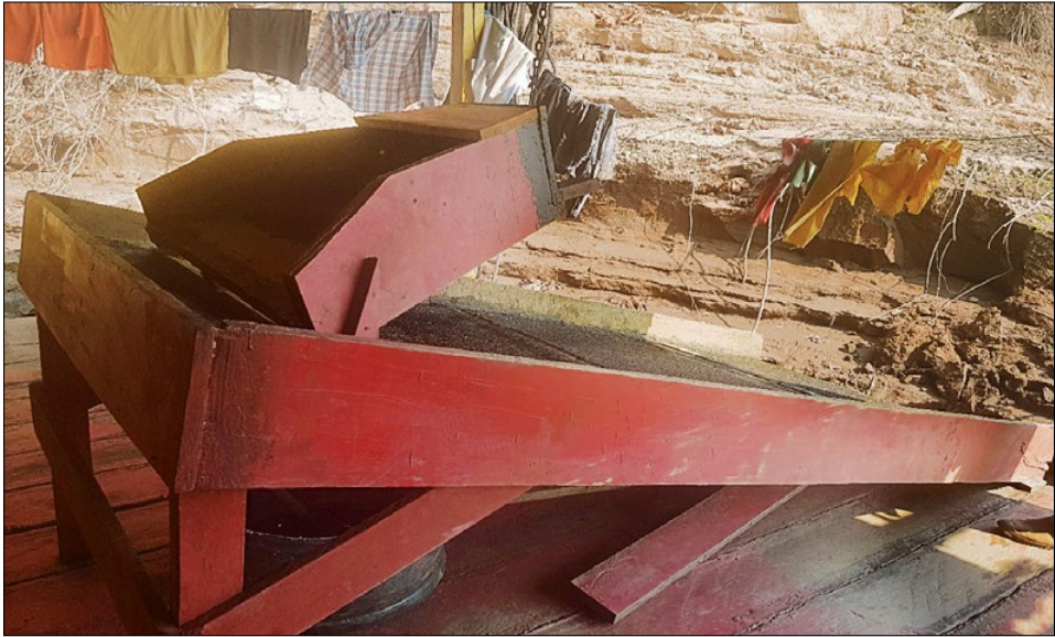
Photo 17 Post-amalgamation secondary gutter to recover fine gold and mercury, Beni (2019).
