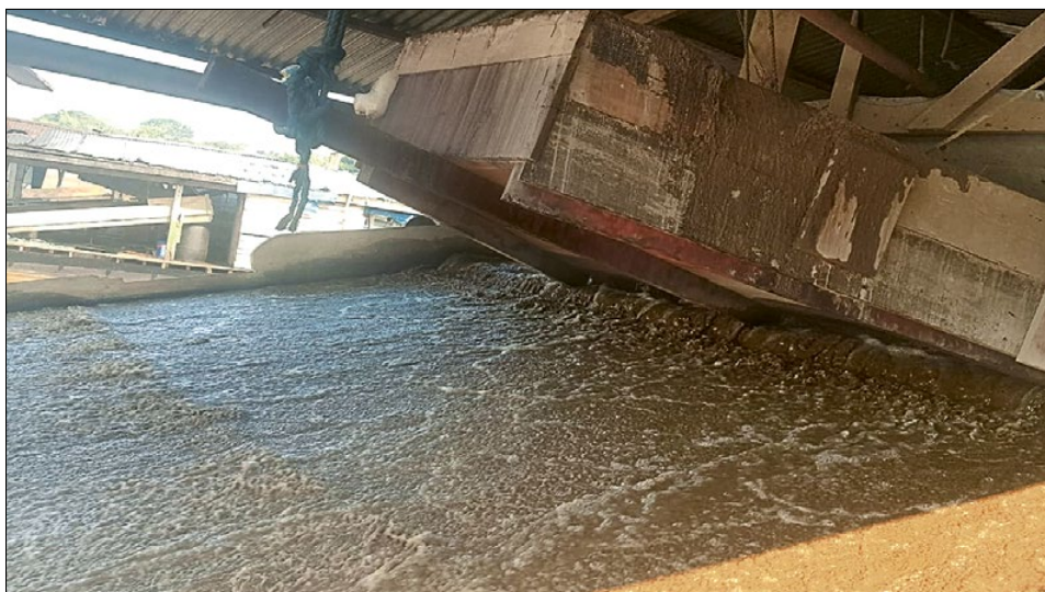
Photo 16 Gutter with carpet for the concentration of alluvial gold in a raft in the Beni river - Beni (2019).
