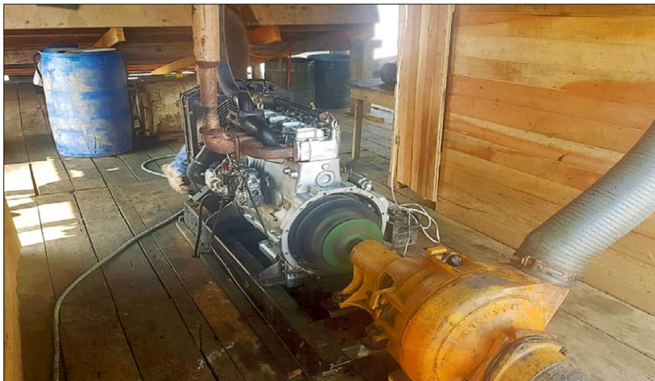
Photo 15 15 MWM engine of 4-cylinders with coupling pads for a 6 x 6 dredge pump (2019).
